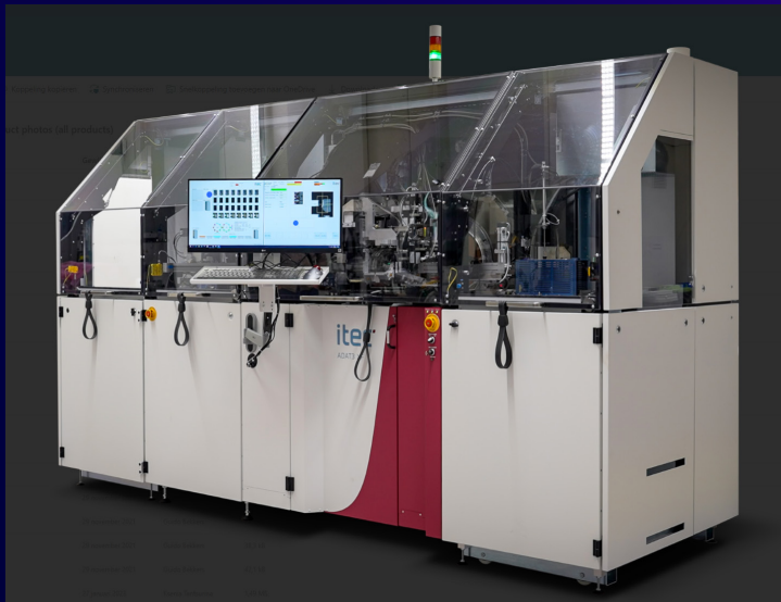
ITEC pick-and-place equipment (ADAT 3 XF)
